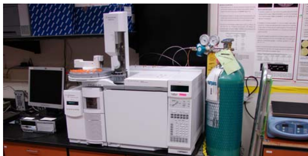
FIGURE 2. DON was quantified using a GC/MS (Agilent 5975 Inert MSD with 6890N Network GC system) operating in EI mode.
